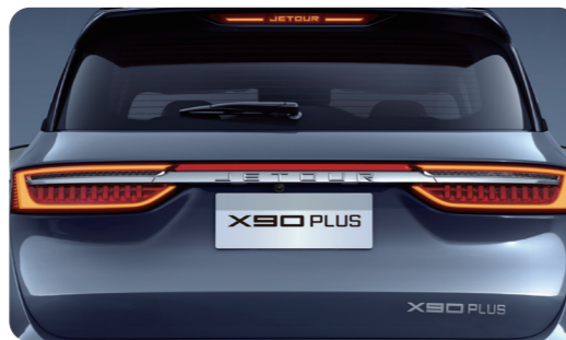
Taillights filled with 236 LED particles
